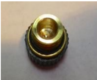
Adjustable Hydrostatic Lubricator cap after being drilled out.
